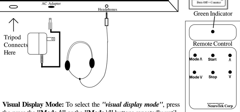
**Visual Display Mode:** To select the "*visual display mode*", press the "Mode Λ" or the "Mode V" buttons repeatedly until all three red dots are on and the left digit displays a "1". When "*visual display mode*" is selected, the right digit will display a "S" for *scan mode* or "E" for *ends only mode*. Press the "Λ" or "V" buttons to switch between "Scan" or "Ends only" modes.
